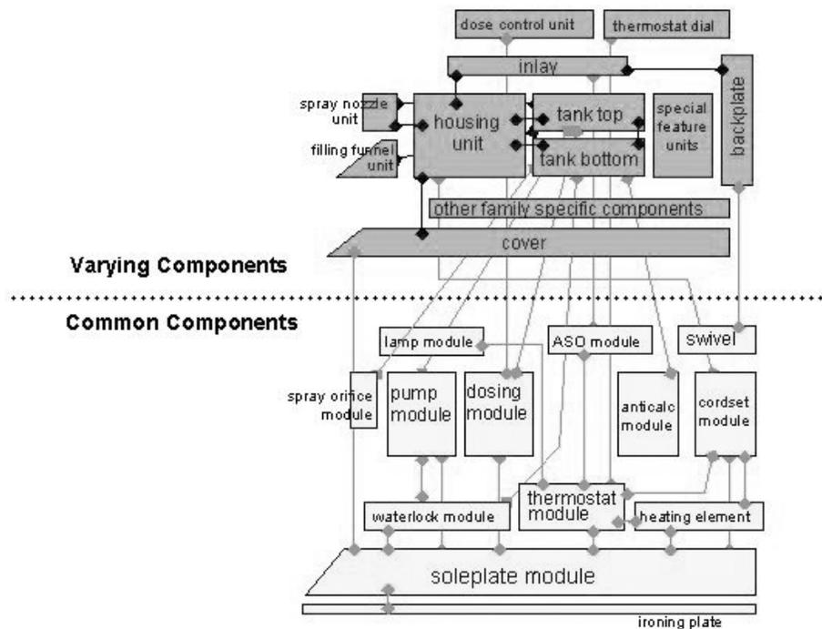
configured by substituting a range of component variations into the architecture without having to make compensating design changes in other components.
