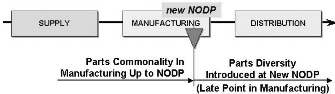
**Figure 5.** Last-point differentiation, National Sales Organizations (NSO) Order Decoupling Point (NODP), in Sunshine platform supply chain (diagram courtesy of Philips Center for Industrial Technology).
